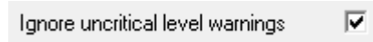
Fig. 114 Checkbox for suppressing the message caused by excessive single level deviation or other uncritical warnings.
