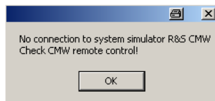
Fig. 130 Missing CMW connection
