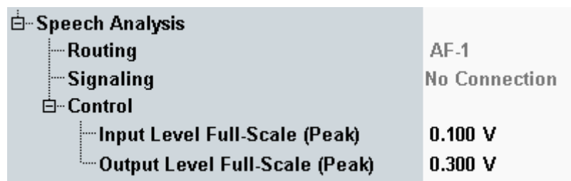
Fig. 57 Setting of the full-scale peak input and output values in the CMW user interface
